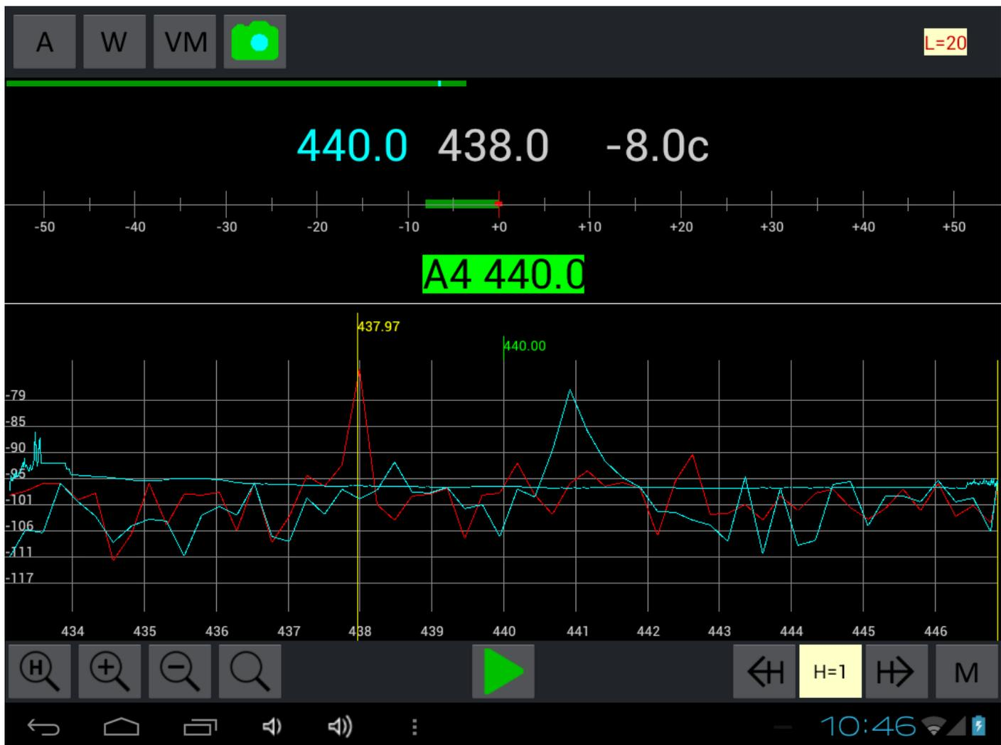
Pressing the button **Snapshot** again resets the spectrum **Snapshot**.
